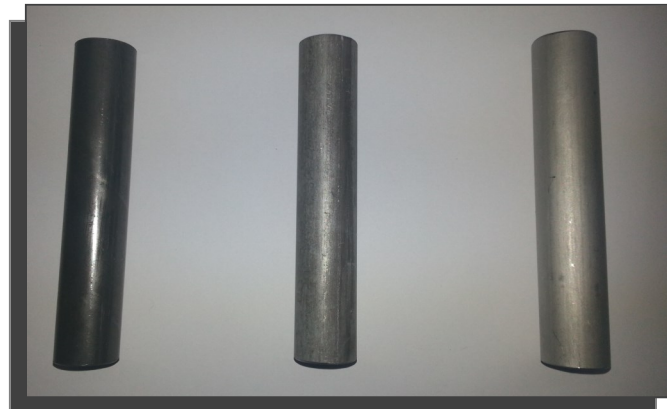
In this picture a raw superduplex tube and the same tube after 2 hours pickling with Descalinox P13 and with Descalinox Fast.
